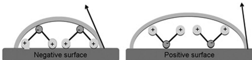
Fig. 4. Schematic representation of the contact angle of negatively and positively surfaces.
